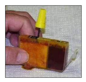
3. Using our Yellow Drill Tool, make a hole in the top of the cartridge into the sponge area.
